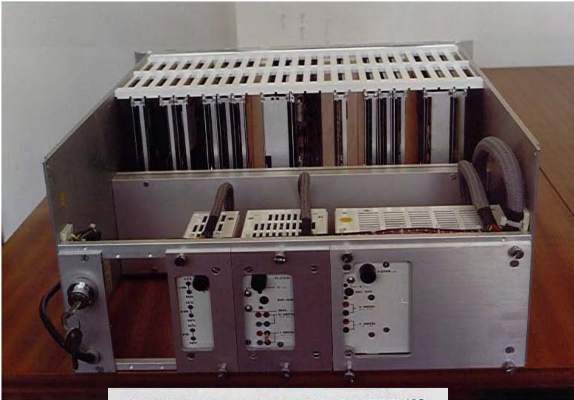
CIMBUS 19" Chassis & CPU, RS 232, IEEE 488, RAM Memory & Floppy Disc Modules
