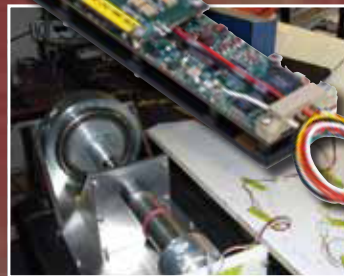
Motor Loading with Oil Immersion for bench test and acceptance of drive and subsystem delivered products.
